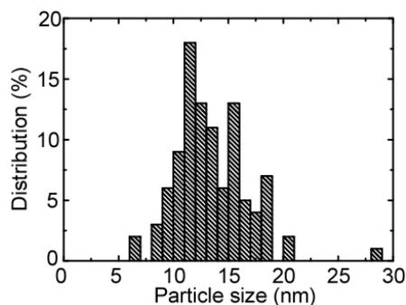
Fig. 2 Size distribution of the fabricated Au NPs.
