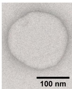
Fig. 3 TEM image of the PC liposome prepared by the negative staining method.
