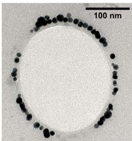
Fig. 5 TEM image for the PCA10 sample by the ultra-thin section method with freeze substitution.
