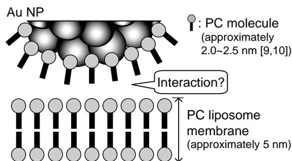
Fig. 6. Structural model for the interaction between the Au NP covered with PC molecules and the PC liposome.
