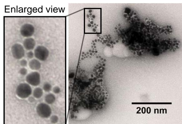
Fig. 4 TEM image for the PCA100 sample prepared by the negative staining method. The enlarged view is also shown.
